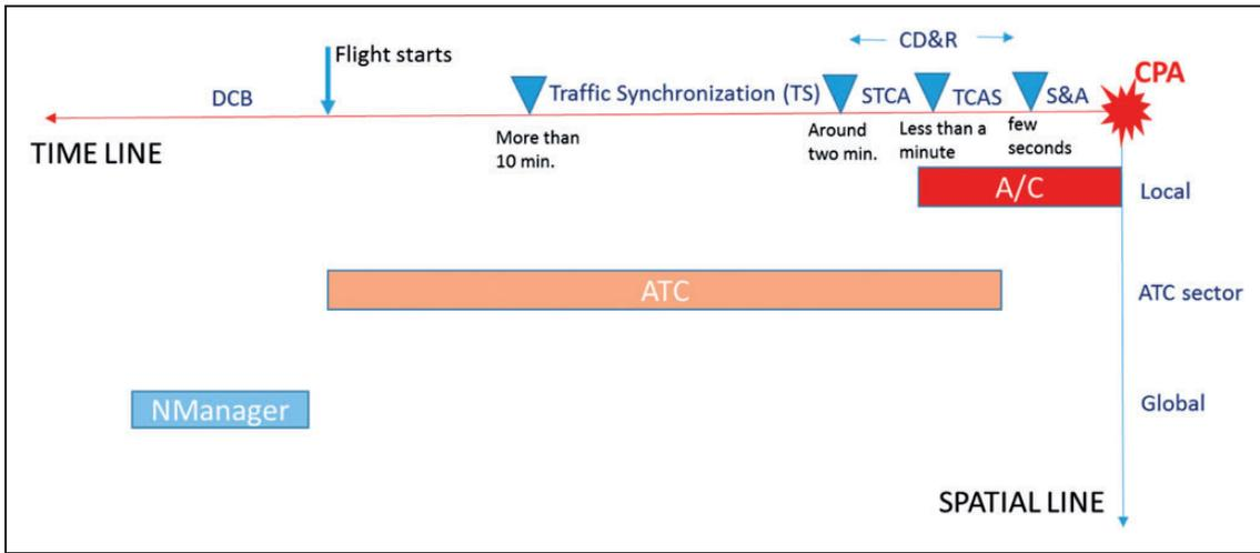
**Figure 8.** ATM resources to avoid separation infringement at “Closest Point of Approach (CPA)” among each aircraft flying within controlled airspace.
