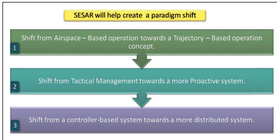
**Figure 1.** The pillars of the shift toward the new ATM system.
