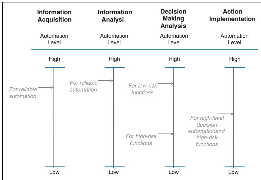
**Figure 4.** Levels of automation for independent tasks. Recommended types and levels for future ATC systems.
