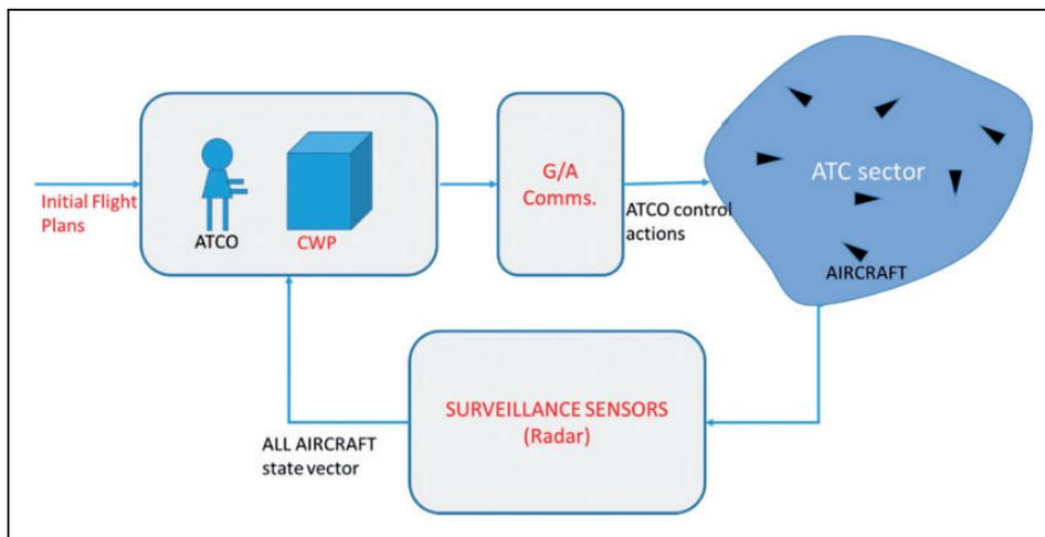
**Figure 9.** ATC sector represented as a single-agent controlled process.
